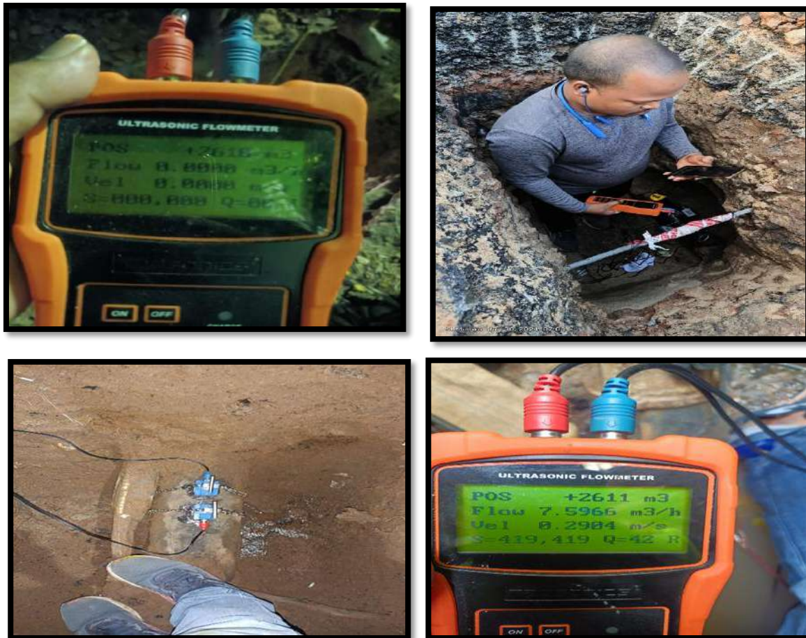
Image 3.15: Flow measurement using Ultrasonic clamp on flow meter
